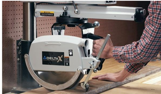
Properly Guarded Saw Blades
