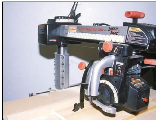
Radial Arm Saw Configured for Ripping – Anti-Kickback Fingers in Place
