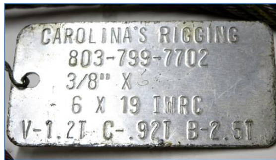
Wire rope sling tag listing capacities measured in tons for various rigging methods. Example not for use in actual lifting applications.
