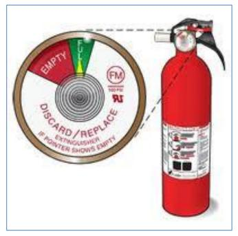
MAKE SURE the needle points into the green "Full" portion of the gauge.
