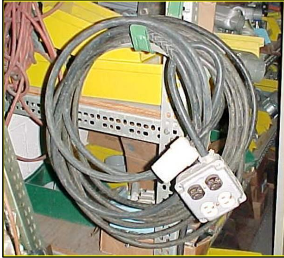
(Electrical outlet boxes used for temporary power supply)
